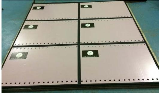
ZIN Technologies developed a light weight tube resonator based technology that provides broad band low frequency noise attenuation called eCALF. ZIN has tested eCALF for both absorption and transmission loss and obtained large attenuation levels especially considering the weight of eCALF.
